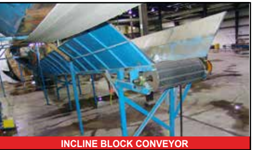
INCLINE BLOCK CONVEYOR
