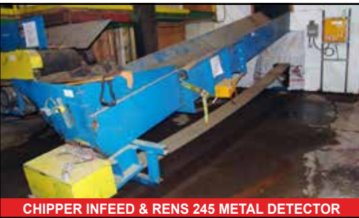
CHIPPER INFEEED & RENS 245 METAL DETECTOR
